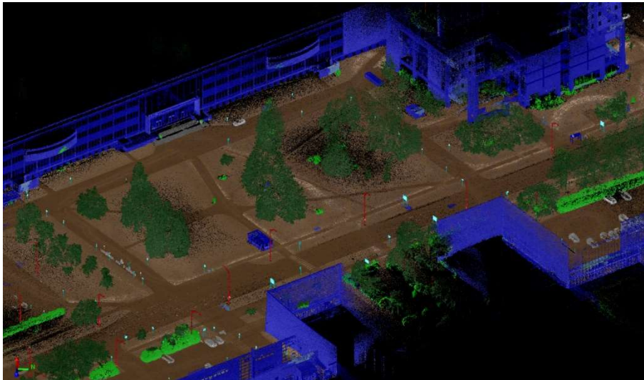
Figure 2 : Point cloud after classification into 11 classes by TBC
