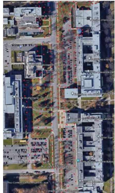
Figure 16 : Simulation of a survey with a tripod-mounted scanner. Each red point represents a station.
