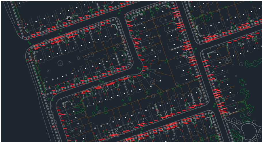
The landbase provides a foundation for FTTH design work. Photo credit Planview USL.
