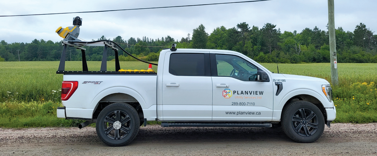
The Trimble MX50 mobile mapping system collects lidar data and 360-degree imagery while driving at posted speeds. Photo credit Planview USL.
